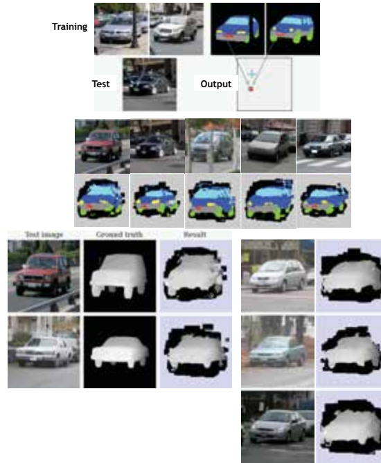
Figure 11.8: As shown by Thomas et al. [2007, 2009a], the ISM top-down segmentation procedure can be generalized to also infer other kinds of meta-data, such as part labels, depth maps, or surface orientations. Based on Thomas et al. [2009a].
