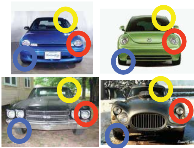
Figure 8.4: While the global object appearance may undergo significant variation inside a category, the appearance and spatial relationship of local parts can often still give important cues. This provides a strong motivation for using part-based models. Courtesy of Rob Fergus and Courtesy of The CalTech256 Dataset.
