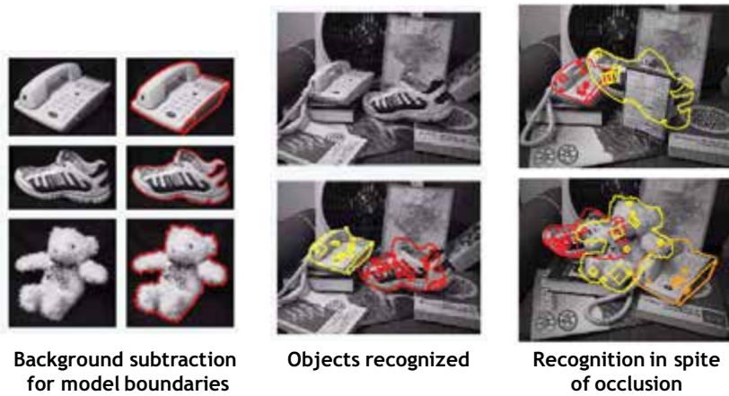
Figure 6.3: Object recognition results with the approach by Lowe [1999, 2004] based on the Generalized Hough Transform. Based on Lowe [1999].
