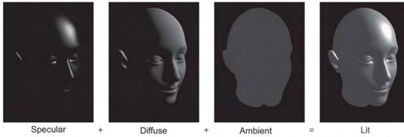
Figure 15.16: The visual contribution of each of the components of the lighting equation
