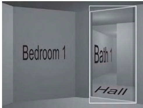
Figure 16.13: The bounding box of a portal polygon
