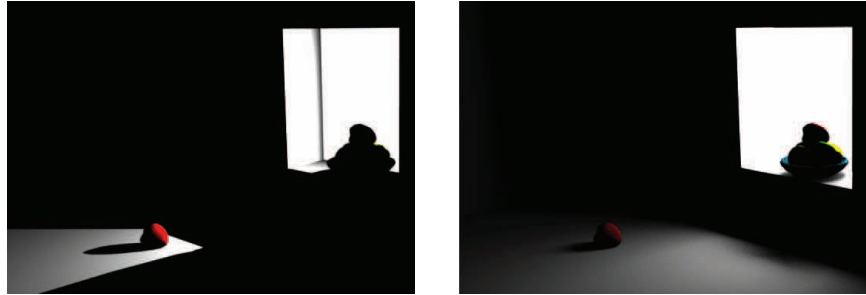
Figure 1.12. This scene shows one example of the importance of soft shadows in obtaining a convincing and realistic-looking scene. On the left is the result using a single hard-shadow sample, whereas the right shows the outcome of a soft-shadow computation.
