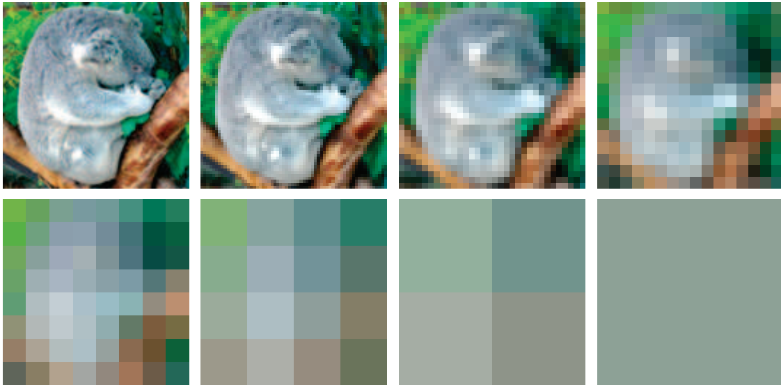
Figure D.2. The mipmap representation is an image pyramid, where each level has its resolution reduced by a factor of four (two along each axis). Four pixels of the previous level are averaged together.
